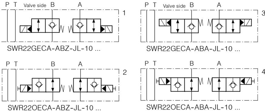
By turning a valve upside down about its short axis, 'Check IN' functions (symbols 1 and 2) become 'Check OUT' functions (symbols 3 and 4)
