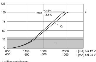
1 = Fine control range 2 = 100% = 2000 ± 200 mA bei 12 V DC 1000 ± 100 mA bei 24 V DC (100%- values vary with nominal flow rate)
