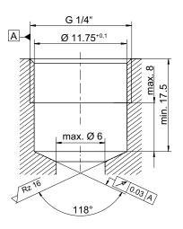
**RVVE-G-06** = check valve / screw-in cartridge valve **REG-03 / REG-04** = dimension of the cavity for screw-in cartridge RVVE-G-06
