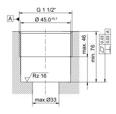
**RVVE-G-40** = check valve / screw-in cartridge valve **REG-03** = dimension of the cavity for screw-in cartridge RVVE-G-40
