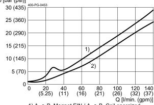
1) A→B, Magnet EIN / A→B, Coil energized 2) B→A, Magnet EIN / B→A, Coil energized
