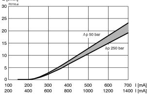
$\Delta p = f(Q)$  Pressure drop - Flow rate characteristic ["200"]  $\Delta p A \rightarrow B$  [bar]
