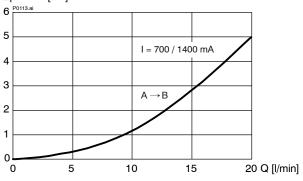
Q = f ( $\Delta$ p; I) Flow rate adjustment characteristic ["200"] Q [/min]
