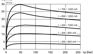
Q = f (I;  $\Delta p$ ) Flow rate adjustment characteristic ["200"] Q [//min]
