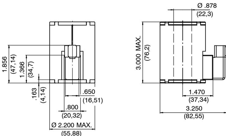
Coil with 1/4" Spade terminals connection, 2-pole
