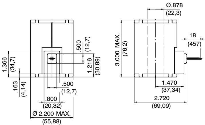
Coil with ISO 4400 / DIN 43 650 connection, 2-pole
